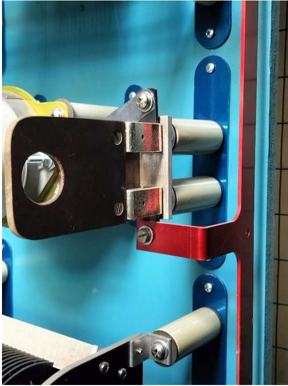
Figure 5 - A portion of a long laser cut busbar at the power division point in our night phasor. This turned out to be an elegant way to strap four J-plugs together.
