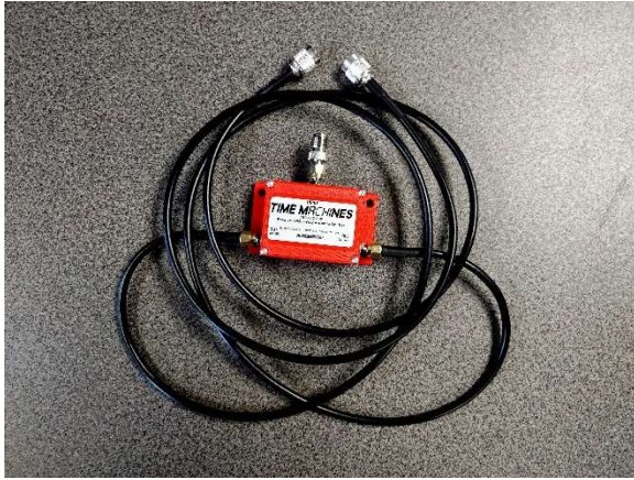
A GPS antenna splitter allowed use of the single rooftop antenna for both exporters.
