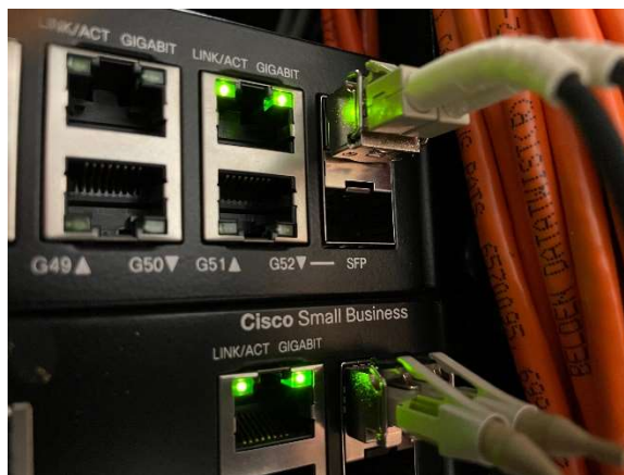
Many switches have combo ports that can be either SFP or wired Ethernet.
