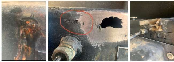
Figure 1 - What started as a pinhole turned out to be much more. Todd made a temporary repair with JB Weld. A permanent repair is pending.
