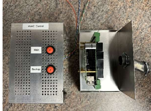
Figure 4 - A work in progress, this Pi-4 and 8-relay HAT will be used for main/backup HVAC control at the KLTT transmitter site.
