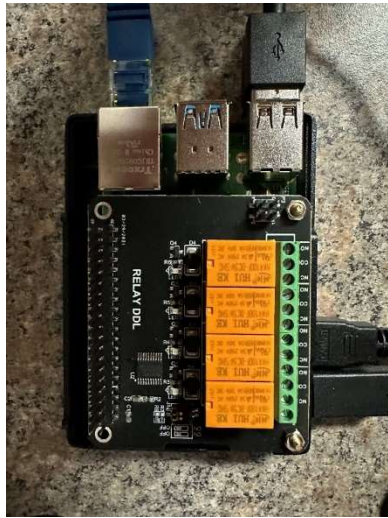
Figure 3 - This Pi-4 and relay HAT is the one we're using in Denver to test SNMP functions for legacy transmitters.
