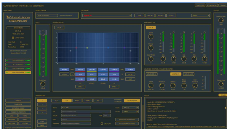
Wheatstone Stream Blade control and monitoring GUI screen.
