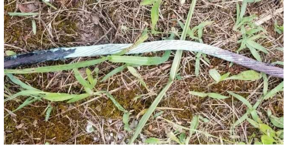
Figure 2 -- One phase at the service entrance got a bit warm.
