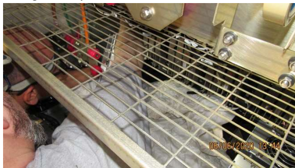
Steve Cuchetti and Nautel's Nelson Bohorquez had to do some contortions to replace the backplane in the WMUZ NX50.
