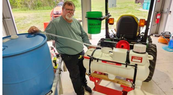
Figure 1 - Chemical sprayer mixes herbicidal concentrate and water on demand.
