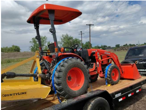
The Kubota secured to the trailer with the new straps and chocks.
