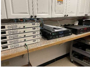
Two Tieline Gateway-8W codecs, two Gateway-4s and five Bridge-IT XTRAs all configured and connected, ready to deploy.
