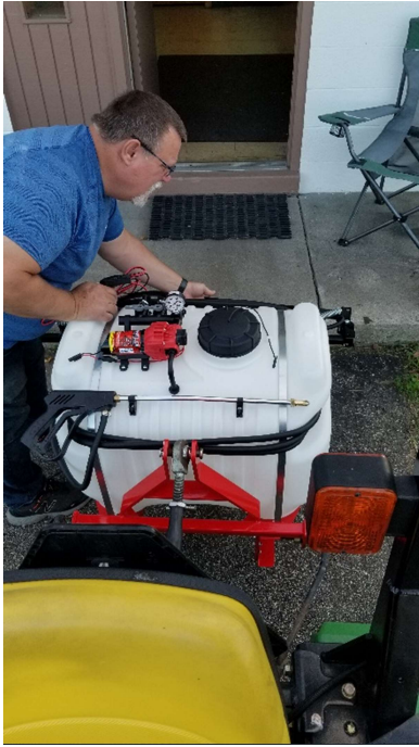
The spray rig attaches to the tractor's 3-point hitch.
