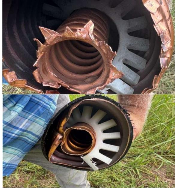
Figure 1 - The two ends of the 200-foot piece of 5-inch line we cut out. Note that the Teflon is clean and bright white in the bottom photo.
