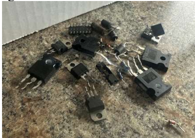
A pile of damaged parts that we replaced in the KLDC J1000.
