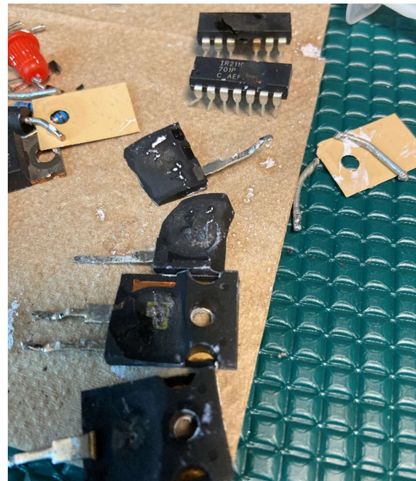
Figure 1 - A LOT of blown-up parts in the power amplifiers of this J1000 transmitter.
