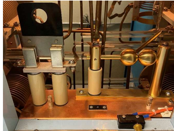
Figure 2 - We now have a properly-spaced and rigidly-mounted ball gap across the transmitter output.
