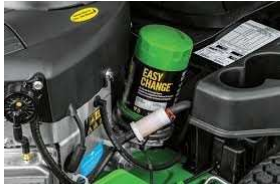
The "Easy Change" oil filter on the John Deere E-120.
