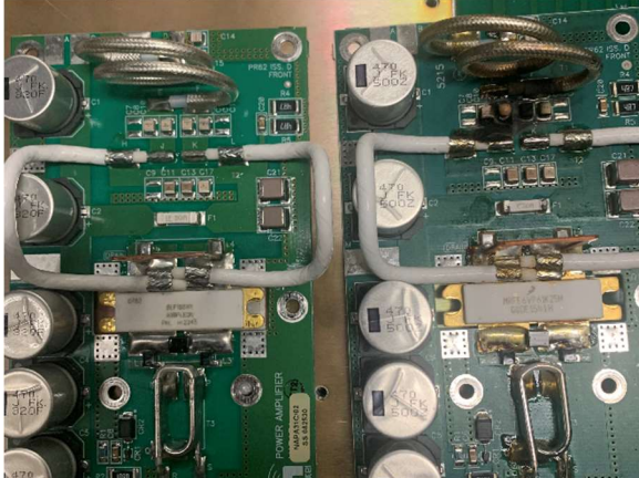
Figure 1 - Some damage is obvious, but both needed to be replaced.
