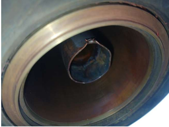
Figure 1 – This flared inner connection, caused by a “split bullet,” was not allowing any power to the top four bays of the antenna.
