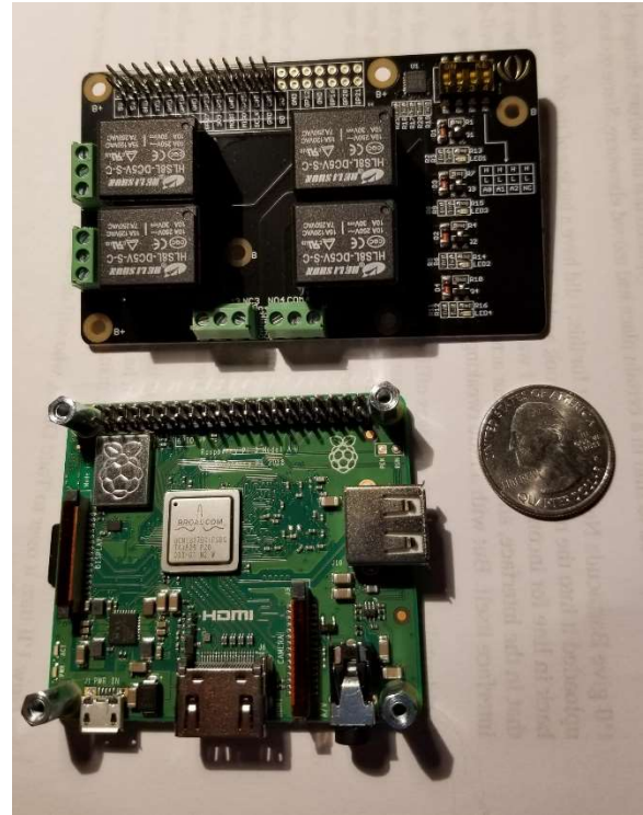
Figure 2 - Raspberry Pi and a Relay “Hat” for contactor control.
