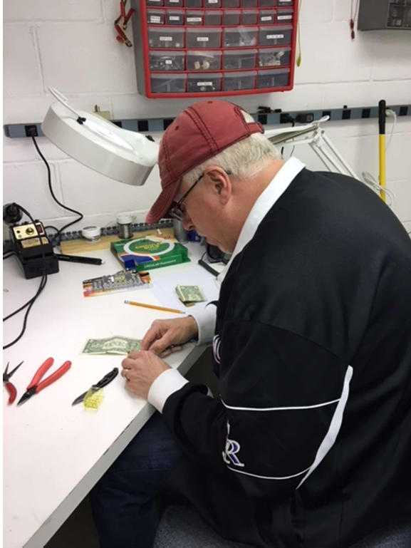
Dad at the workbench at the KLTT site cleaning a relay. He used a dollar bill to burnish the contacts.
