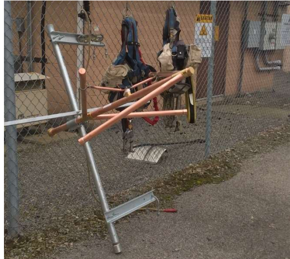
The WDCX(AM) 107.1 MHz translator antenna, assembled and ready to hoist.
