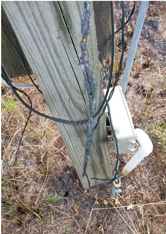
Figure 1 - Lightning did a bit of damage to WXJC-FM's phone line in July.
