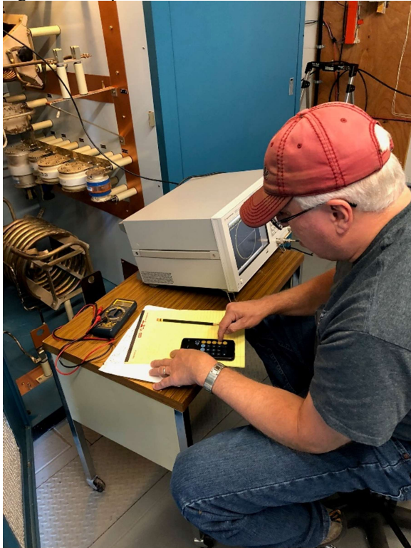
Figuring out the electrical length of a transmission line from the zero crossing frequencies.
