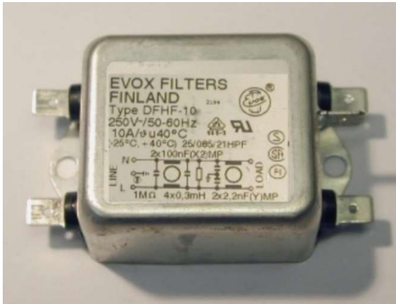
Figure 2 - A standard AC filter works fine on a POTS line.
