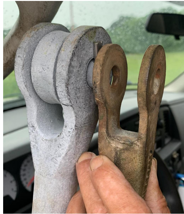
Figure 4 - The clevis on the replacement rod was a wee bit too big.
