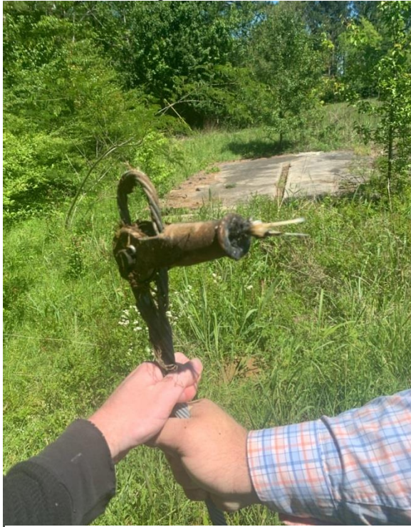
Figure 1 - This is what was left of the fiberglass rod on tower #5.
